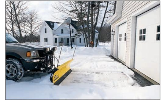
Exclusive Scrape Lock feature hydraulically locks the blade down for clean scraping action.
