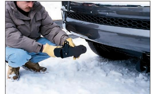
The receiver brackets on your vehicle are removable, by simply pulling the pins, for optimum ground clearance when you're not plowing.
