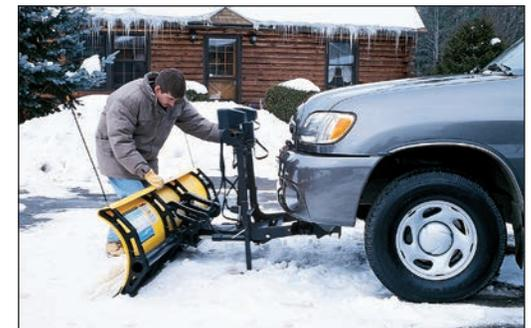
Attaching your Homesteader snowplow is so simple. Either drive into the attachment arms on the plow, or slide the Homesteader into the receiver brackets on your vehicle. Then connect two pins, remove two jacks, and plug in the electrical connectors.
