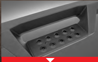
Heavy duty punch plates for high traction step areas
